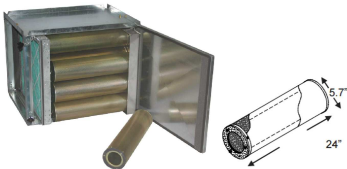
Figure 3. Camfil radial flow HVLA housing architecture and nominal cartridge dimensions (in). Eight cartridges were installed in the housing.
