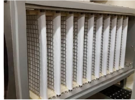
Figure 7. View of SMF with pleat screen supports.
