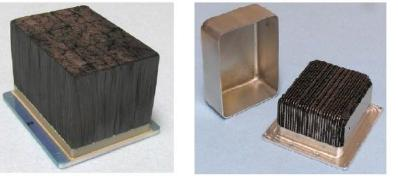
Core material helps to spread heat uniformly throughout assembly. Void areas of core are filled with PCM. PCM generally stays in contact with core
