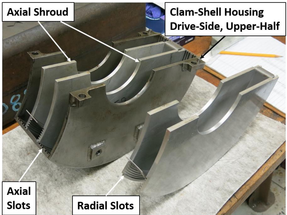
Figure 4 – Configuration of axial and radial shrouding using machined slots. Axial shrouds are 0.25 in. (6.35 mm) thick.
