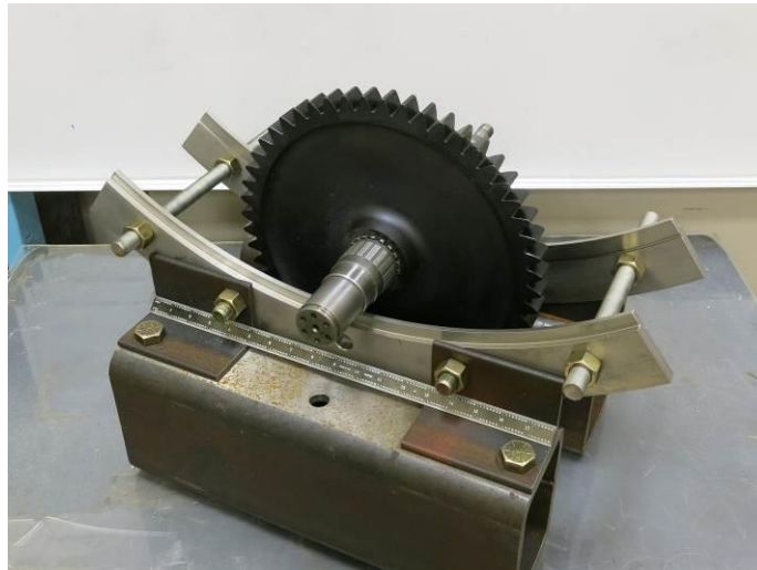
Figure 7 – Example experimental setup for tare loss calculation using curved rail method.
