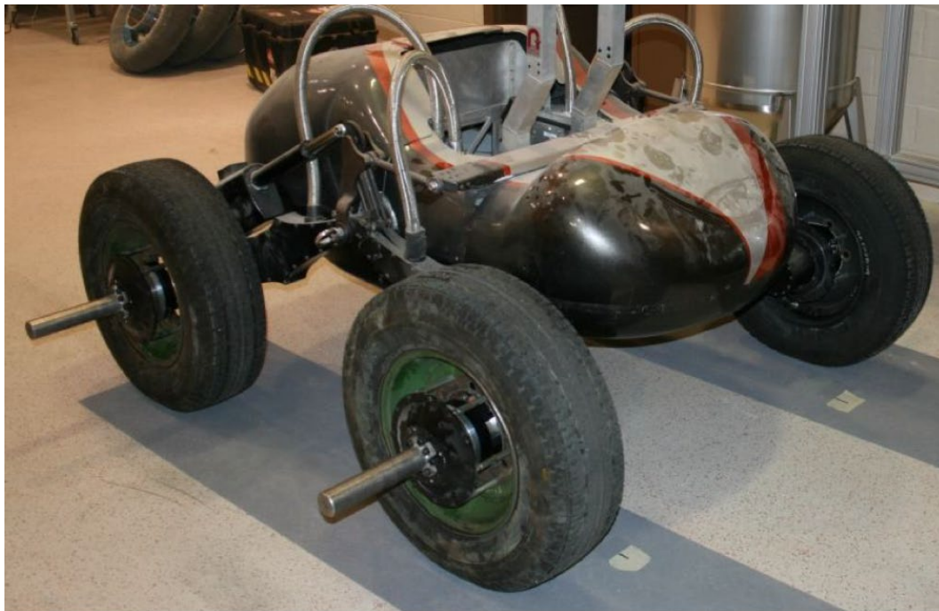
Figure 25.—Scarab rover with rubber treadless pneumatic tires.
