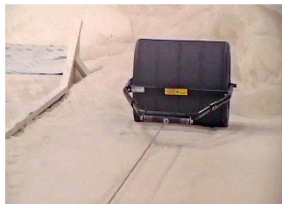
Figure 15.—Soil compacted with a 24-in. lawn roller pulled down the test lane via a mechanical winch.
