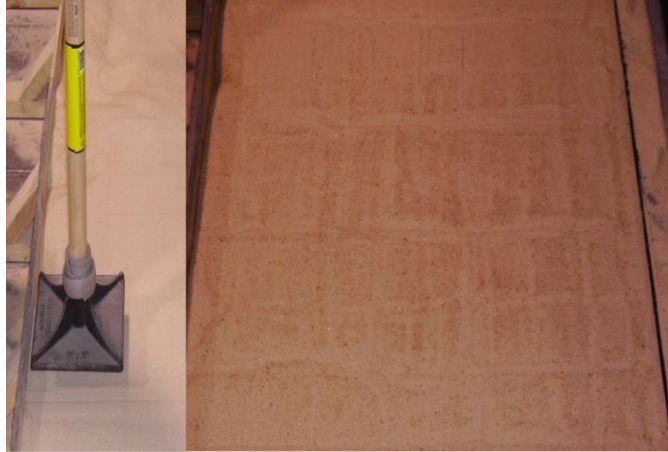
Figure 30.—Terrain compaction produced by dropping an 8- by 8-in. (20.3- by 20.3-cm) tamper from a specific height in an overlapping pattern (tamping method discussed in Section 2.4.2).
