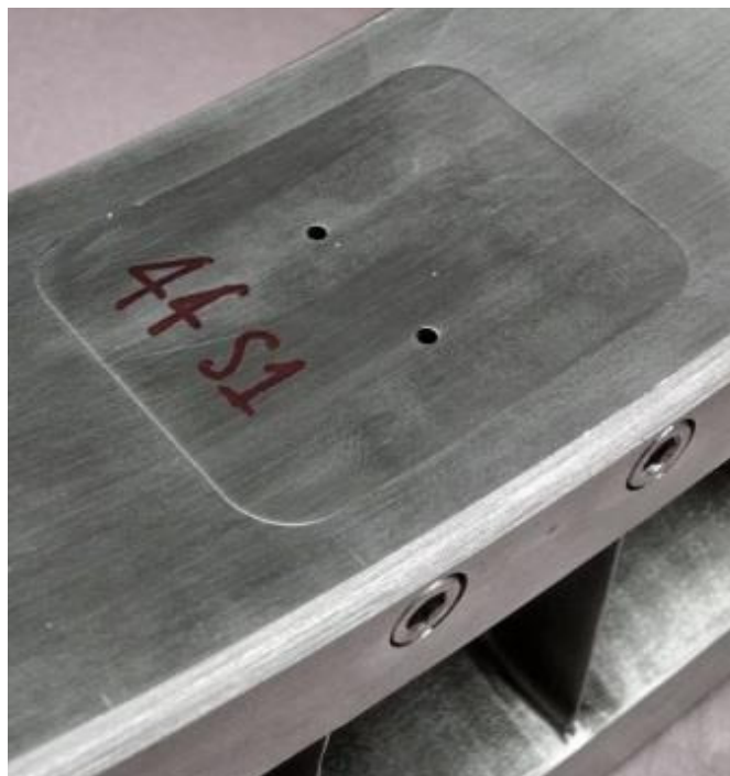
Figure 2.13: Photograph of removable sensor block installed in stator hub shroud.
