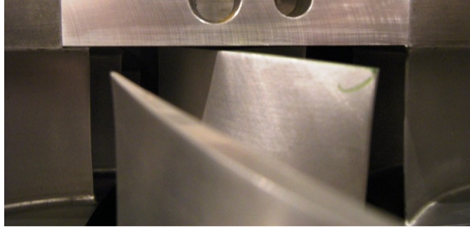
Figure 2.4: Missing 45 degree ramp upstream of Rotor 2, shown here for TC2. Flow is from left to right.
