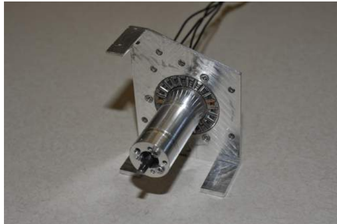
Figure 4: Sleeve Attaches To Motor for Later Mounting
