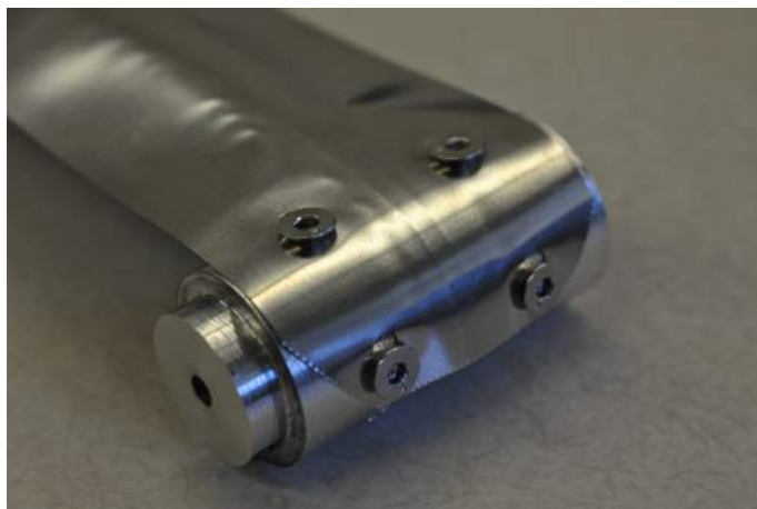
Figure 3: Boom is Secured to Drum
