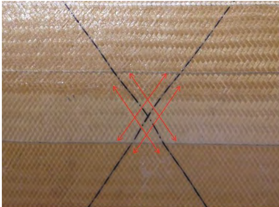
Figure 9. Braid fabric directions.
