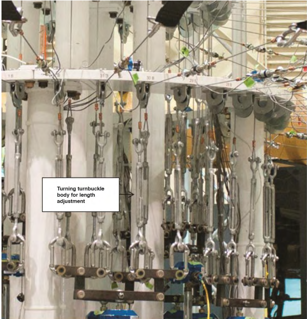
Figure 55. Turnbuckle adjustments were made to provide more available jack stroke.
