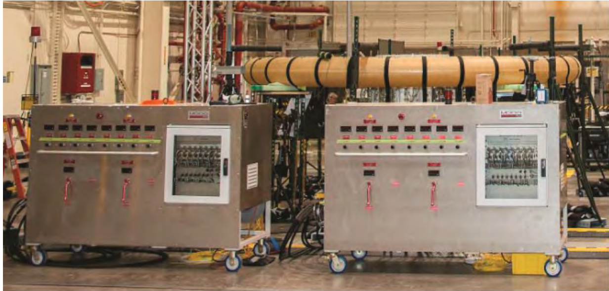
Figure 22. The hydraulic carts used for hydraulic actuator control.
