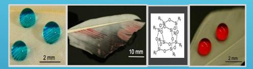
Duck feather repels water (blue), but not oil (red). Surface become omniphobic after dipcoated in a solution of fluorodecyl POSS.
