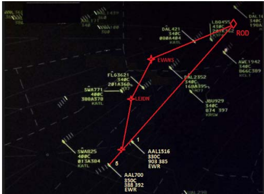
Figure A-3: Example path stretch using automatically selected, named waypoints
