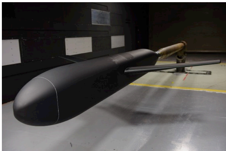
6% Juncture Flow Model in the LaRC 14'X22' Wind Tunnel Nov/Dec 2015
