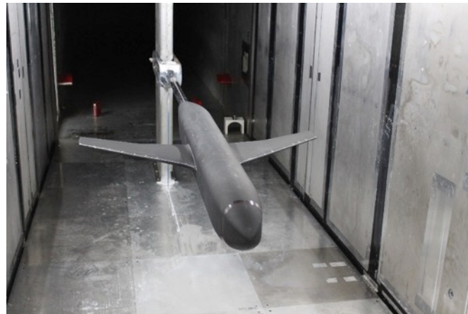
2.5% Juncture Flow Model in the VA Tech 6-foot Stability Wind Tunnel Aug 2015 Model loaned to VA Tech for further testing and educational use
