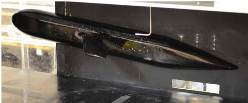
3% Semi-span Juncture Flow Model in the ARC Fluid Mechanics Lab Jun 2015 Model loaned to Caltech for Boeing/Caltech test
