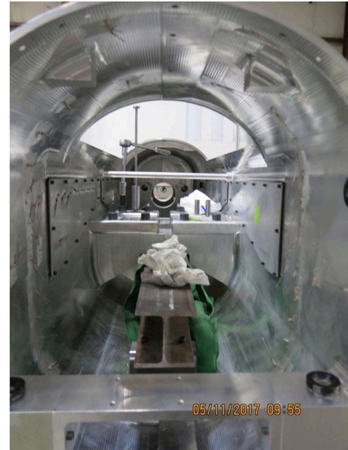
8% Juncture Flow Model for LaRC 14'X22' Wind Tunnel test (first entry Nov 2017)
