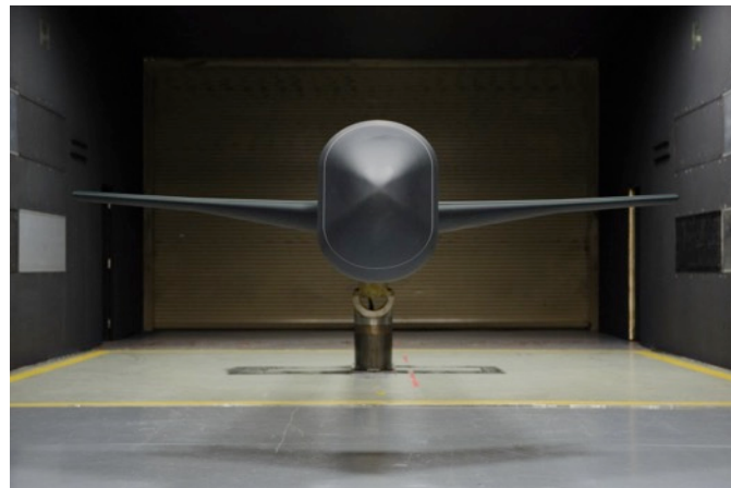
6% Juncture Flow Model in the LaRC 14'X22' Wind Tunnel Nov/Dec 2015
