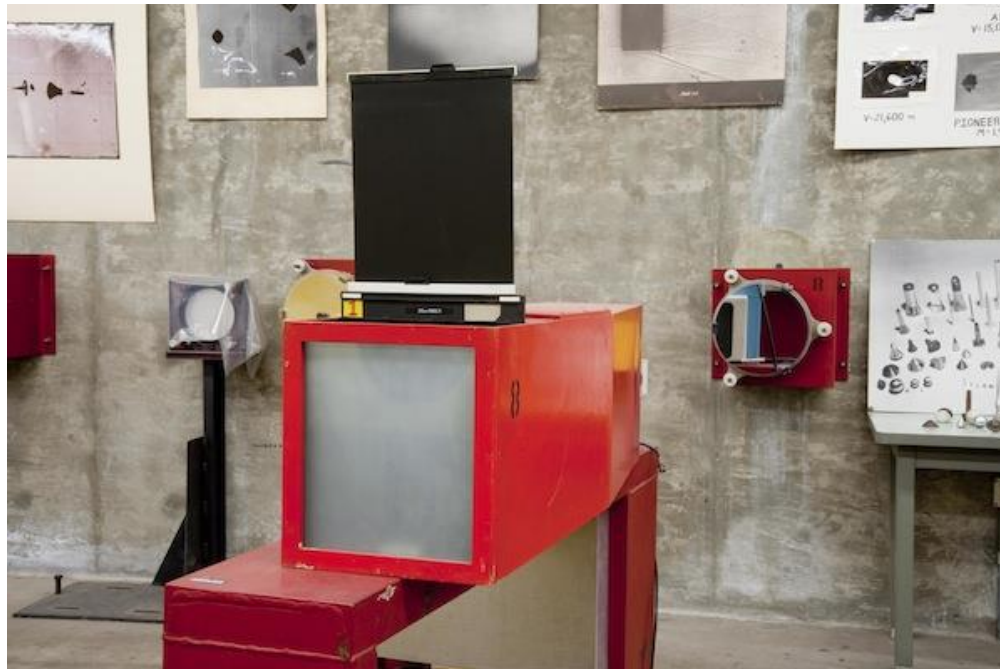
Fig. 9. An original horizontal shadowgraph camera station, looking south. Red film box is in foreground, hiding the Kerr cell assembly. The focusing mirror is in the background.
