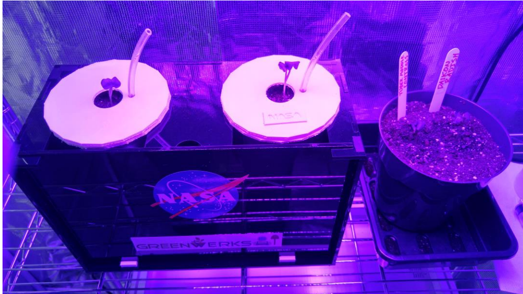
Figure 14. Prototype growth test: top view. Module plants (left) and control plants (right) immediately after transplant
