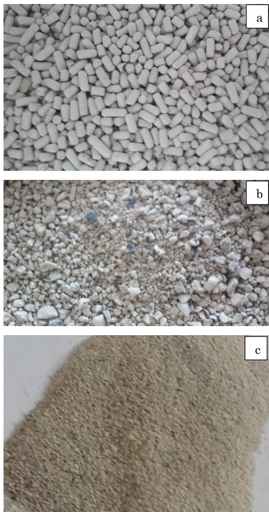
Fig. 1 – Mechanical separation of zeolite: a) zeolite granules before separation, size ~ 3.6 mm; b) zeolite particles after grinding, sizes from 1 micron to 1 mm; c) zeolite particles after sieving, sizes 1 to 250 microns
