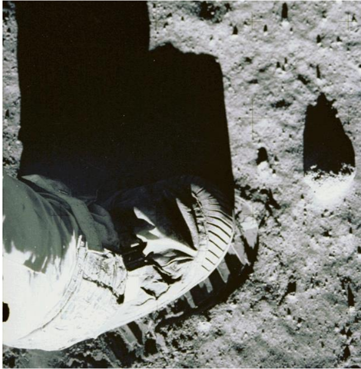
Figure 4. Close up view of the lunar regolith with Apollo 11 astronaut Edwin “Buzz” Aldrin’s boot for scale, showing consistency of the uppermost surface (NASA image AS11-40-5880).
