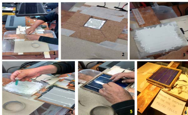
Figure 8: 1) Application of lower face of Peltier Cell to the heat sink; 2) Thermal insulation and conductive paste on Peltier cell; 3) Aluminum plate and conductive paste; 4) Application of conductive paste for the electrical link between Al. plate and PV cell; 5) Application of PV cell; 6) Workbench
