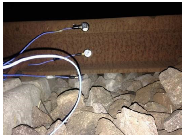
Figure 8 : Accelerometers positioned on the rail
