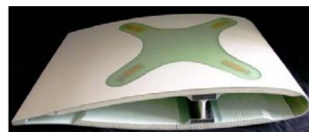
Fig. 7: Embedded PZT fiber transducer
