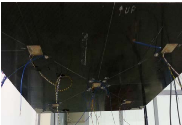
Fig. 1: Piezoceramic patches bonded on the panel
