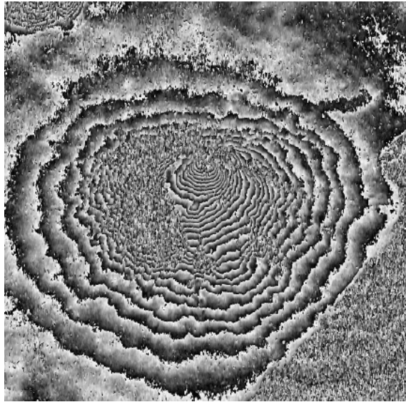
Figure 1: These fringes based on the radar phase measurements can be interpreted as topographic contours for the area around Vesuvius. The image was obtained by combining two ERS SAR images interferometrically [1].
