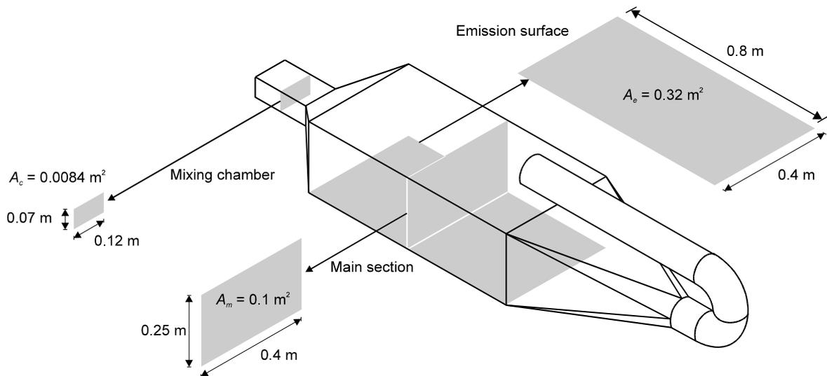
Figure 2 Schematic of wind tunnel and dimensions
