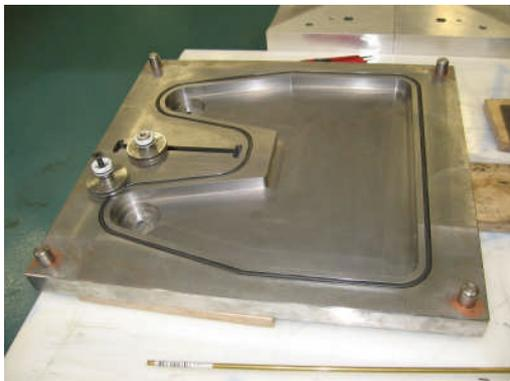
Figure 6. RTM mould tool base with hole inserts
