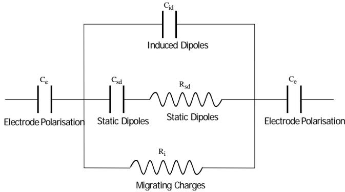
**Fig. 1** Equivalent circuit representation of the electrical response of thermosetting materials
