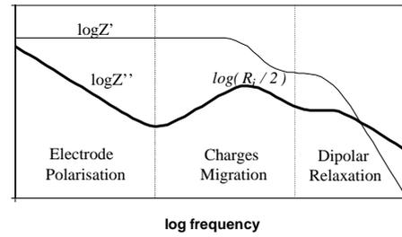
**Fig. 2** Impedance spectrum of the electrode polarisation-charge migration-dipolar relaxation circuit
