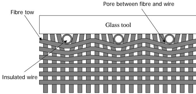
**Fig. 3** Sensing configuration for flow monitoring in carbon reinforcements
