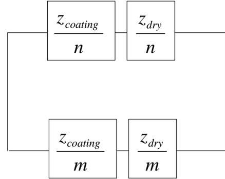
**Fig. 4** Equivalent circuit representing the response of the flow sensing setup
