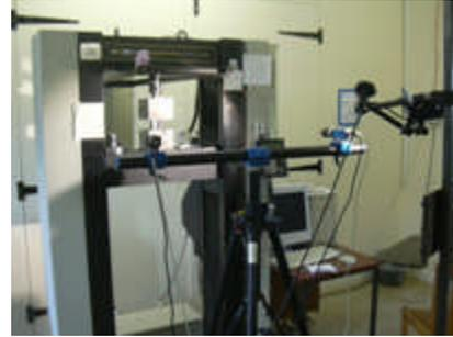
(b) Optical strain measurement set up
