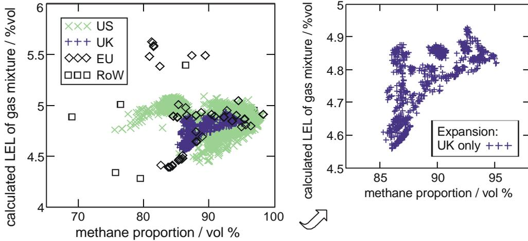
Figure 5. Illustration of the range of calculated true LELs for the gas mixtures used in this study, plotted as a function of the proportion of methane in the mixture.
