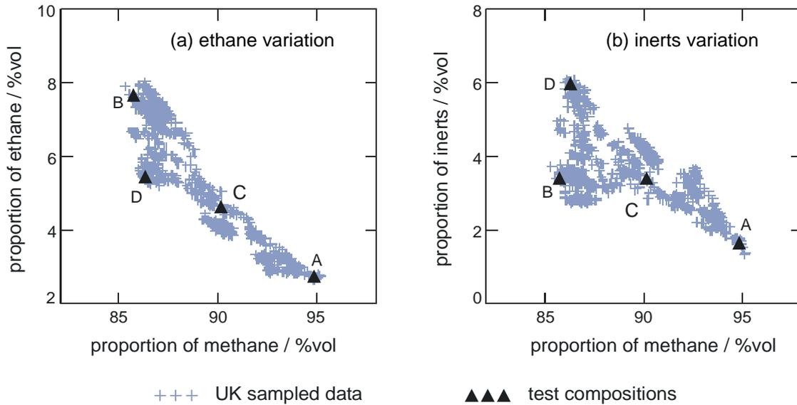
Figure 2. Proportions of ethane and total inerts ( $\text{CO}_2$  plus  $\text{N}_2$ ) versus methane proportion, for test gas compositions and the UK composition data used elsewhere in this paper.
