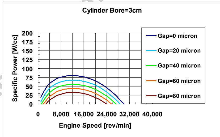
Figure 3b: The corresponding specific brake engine power.
