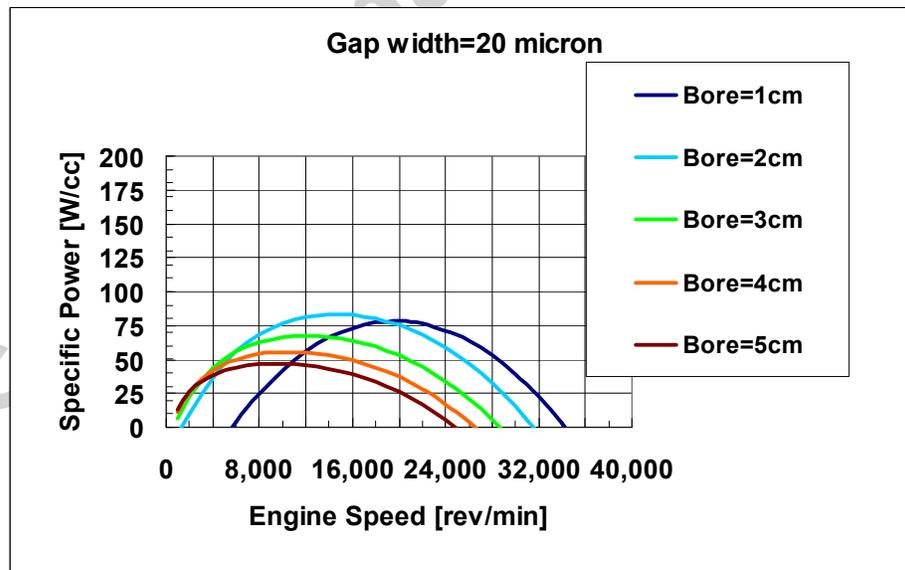
Figure 4b: The corresponding specific brake engine power.
