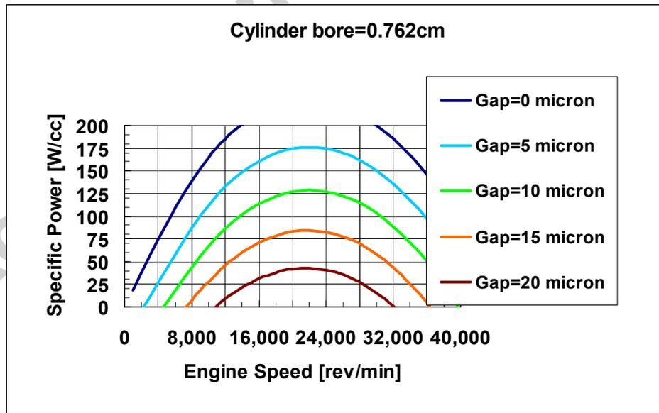
Figure 6b: The corresponding specific brake engine power.
