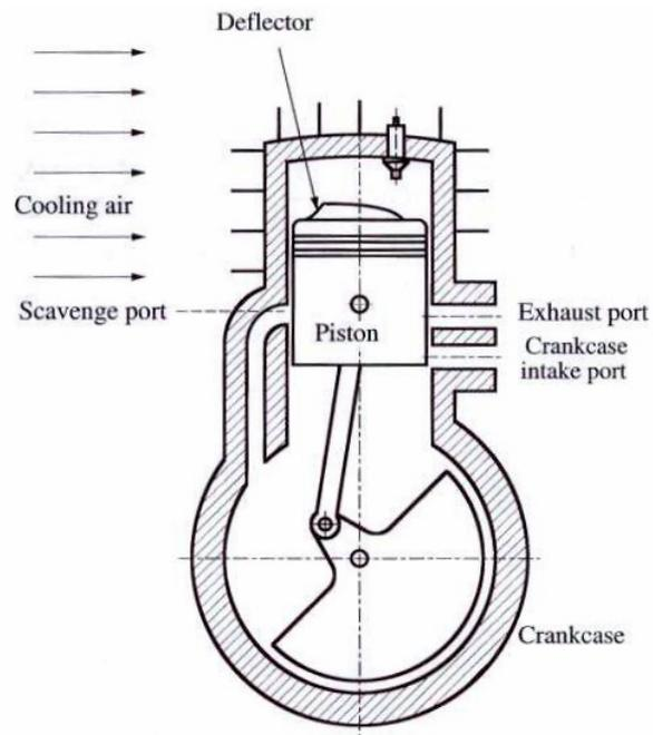
Figure 1: A schematic sketch of a simple SI crankcase-scavenged (Schnurle type) two-stroke engine<sup>18</sup>.
