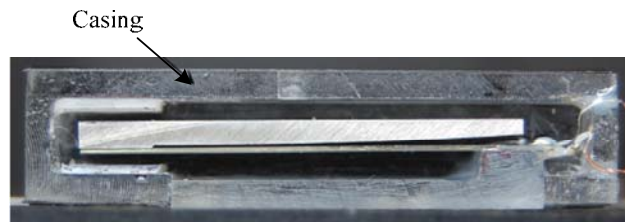
Figure 2-29 Photograph of the rectangular piezoelectric cantilever with L-shaped mass [129].
