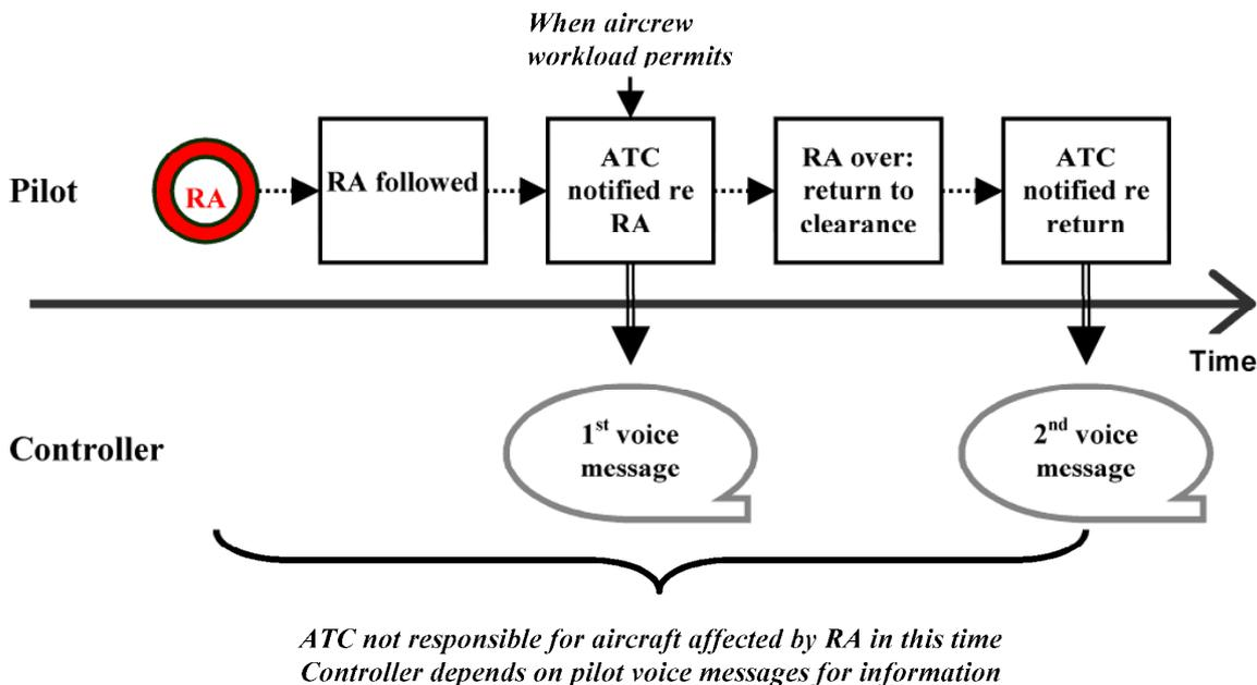
**Figure 3** *Desired sequence following an RA – simplified*
