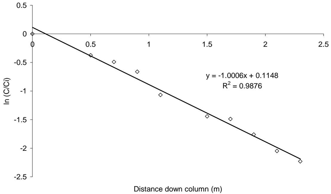
Figure 7: Logarithmic suspended solids removal profile using 2.5-4.5 mm StarLight with a flow rate of 0.4 l/min
