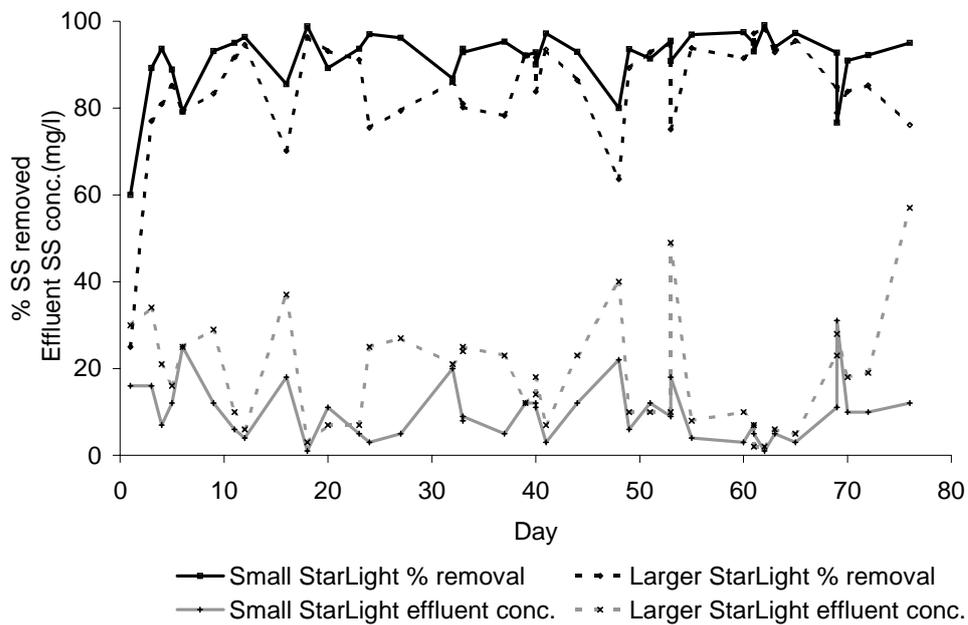
Figure 1: Suspended solids (SS) removal performance during operation
