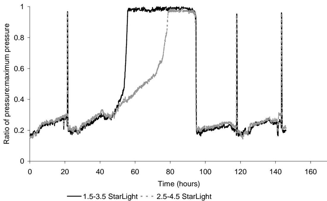
Figure 6: Pressure development with a flow rate of 0.4 l/min
