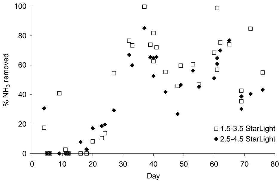
Figure 4: % removal of ammoniacal nitrogen (NH<sub>3</sub>) during operation
