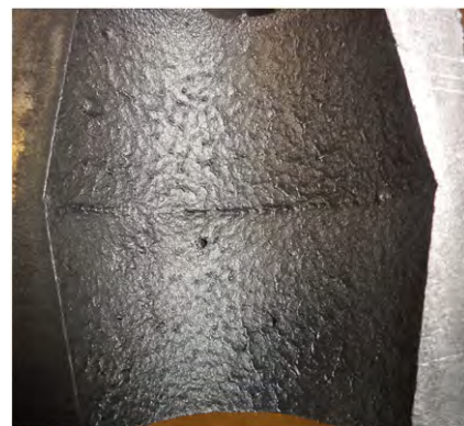
Fig. 13. The surface appearance of a casting made with 50% solid content.
