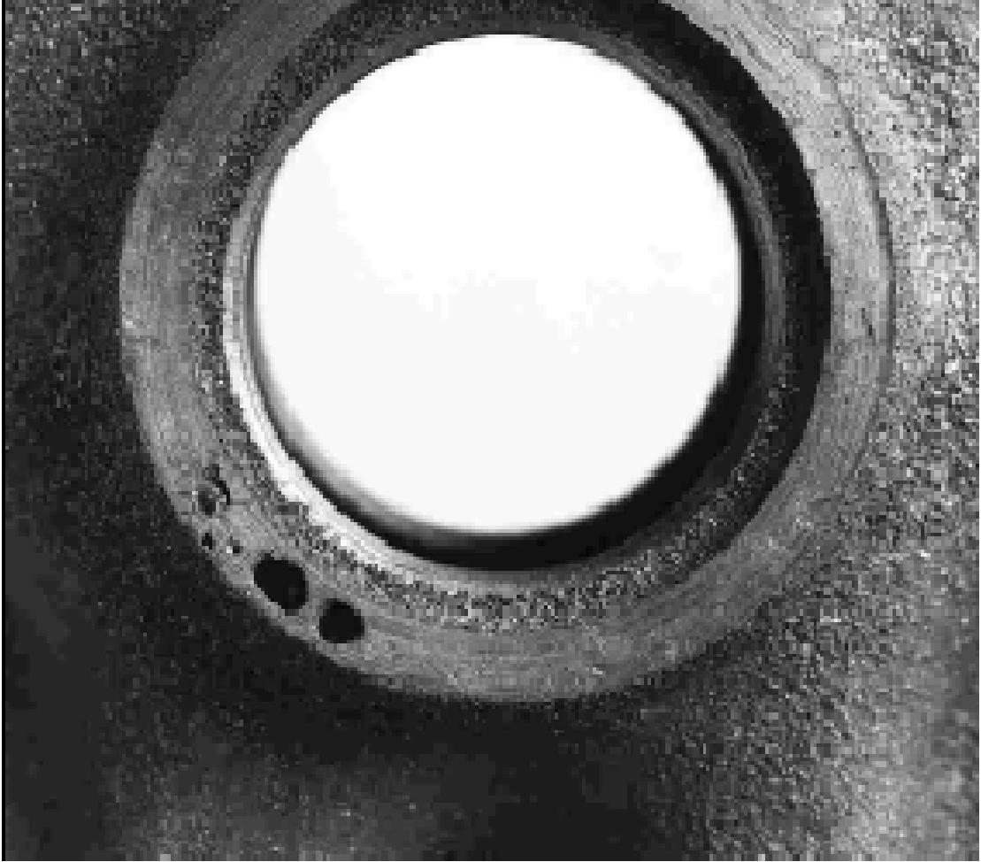
Figure 2.18: Blow holes defects [70].
