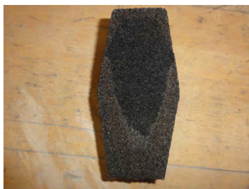
(f) Furan core dip-coated for 5s
