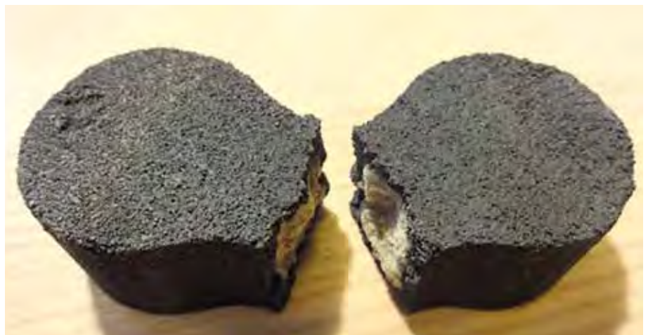
Figure 9: Broken dog bone specimen subjected to uniaxial loading in new STM
