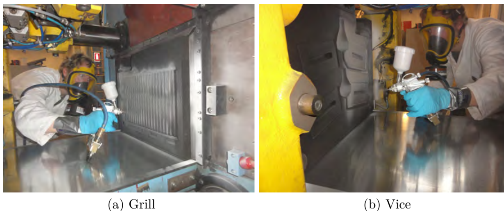
Figure 5.7: The spray-coating process of green sand moulds.
