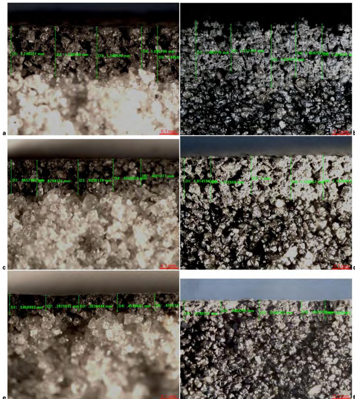
a 40% on cold box; b 40% on furan; c 50% on cold box; d 50% on furan; e 60% on cold box; f 60% on furan 10 Stereofractographs showing effects of solid content on penetration of cold box and furan at 5 s dip coating
