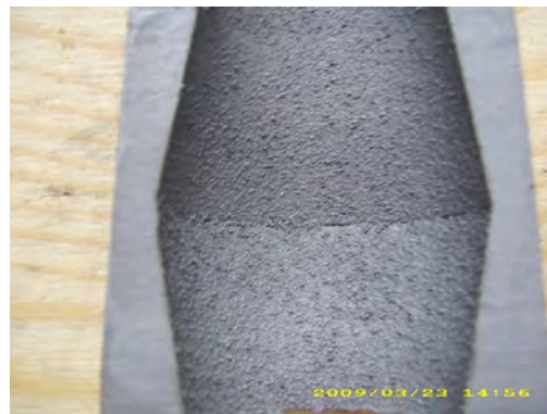
(f) Furan core dip-coated for 5 s
