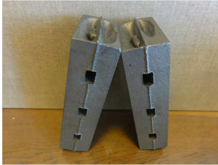
Figure 6.36: Experimental casting showing areas of defects in agreement with numerical simulations in the vertically-parted mould.
