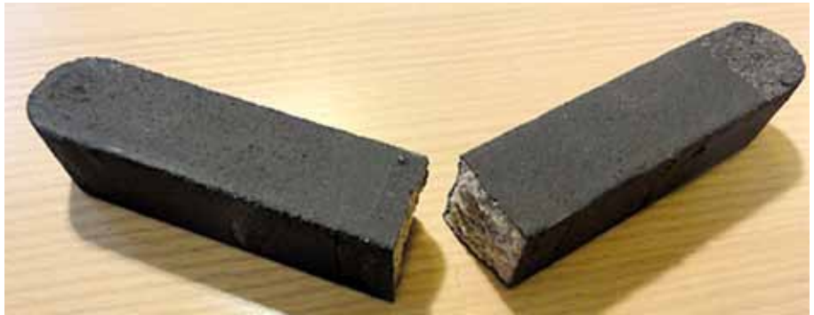
Figure 12: Broken bar specimen subjected to bending test in new STM
