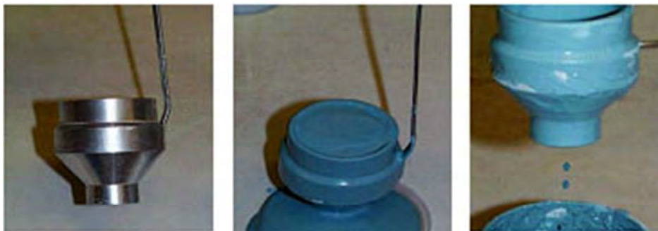
Figure 8. Measurement of viscosity with a Flow cup [45].
