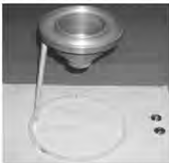
Fig. 1 Ford cup 4 used for measuring the viscosity of the coatings
