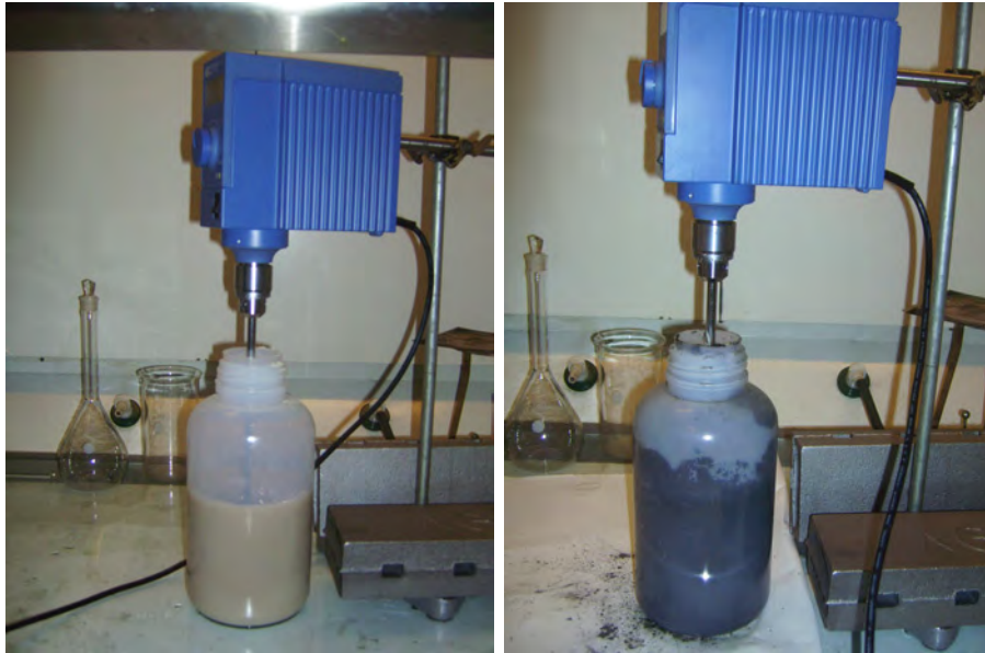
(a) mixing sol-gel component and bentonite (b) mixing after adding filter dust
