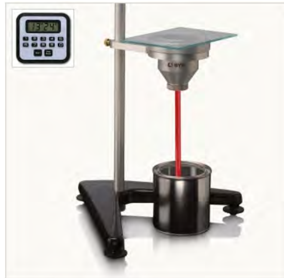
Figure 5.6: Measurement of viscosity by efflux time [99].
