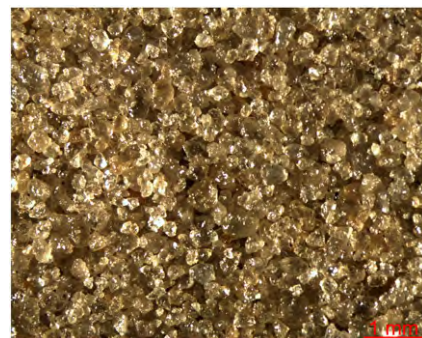
Fig. 6. Surface of uncoated PUCB core showing the sand grains.
