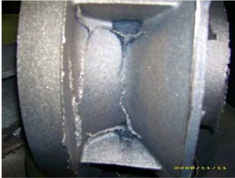
Figure 2.11: Veining or finning and sand burn-on defects on casting surface.
