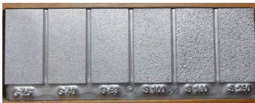
Fig. 3: Tactile comparators for casting surface roughness after shot blasting (Sweden).
