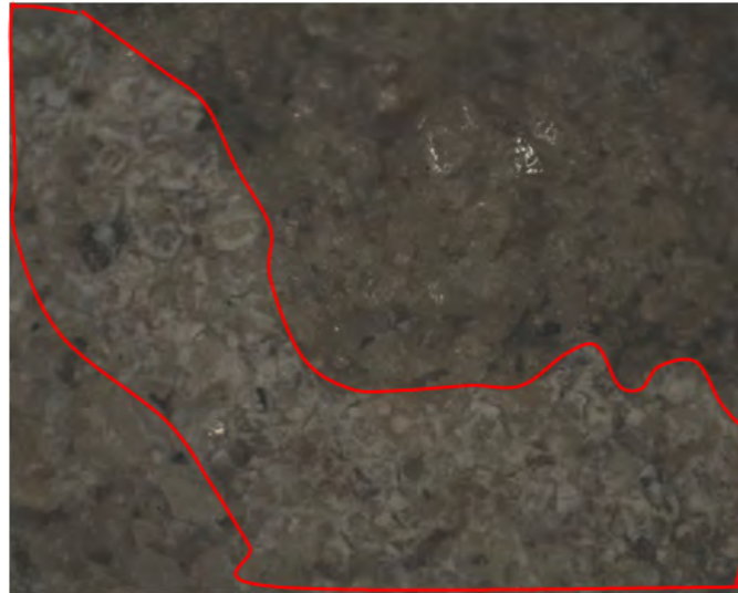
Figure 6.4: Agglomeration of the nanoparticles in the bulk of the core.
