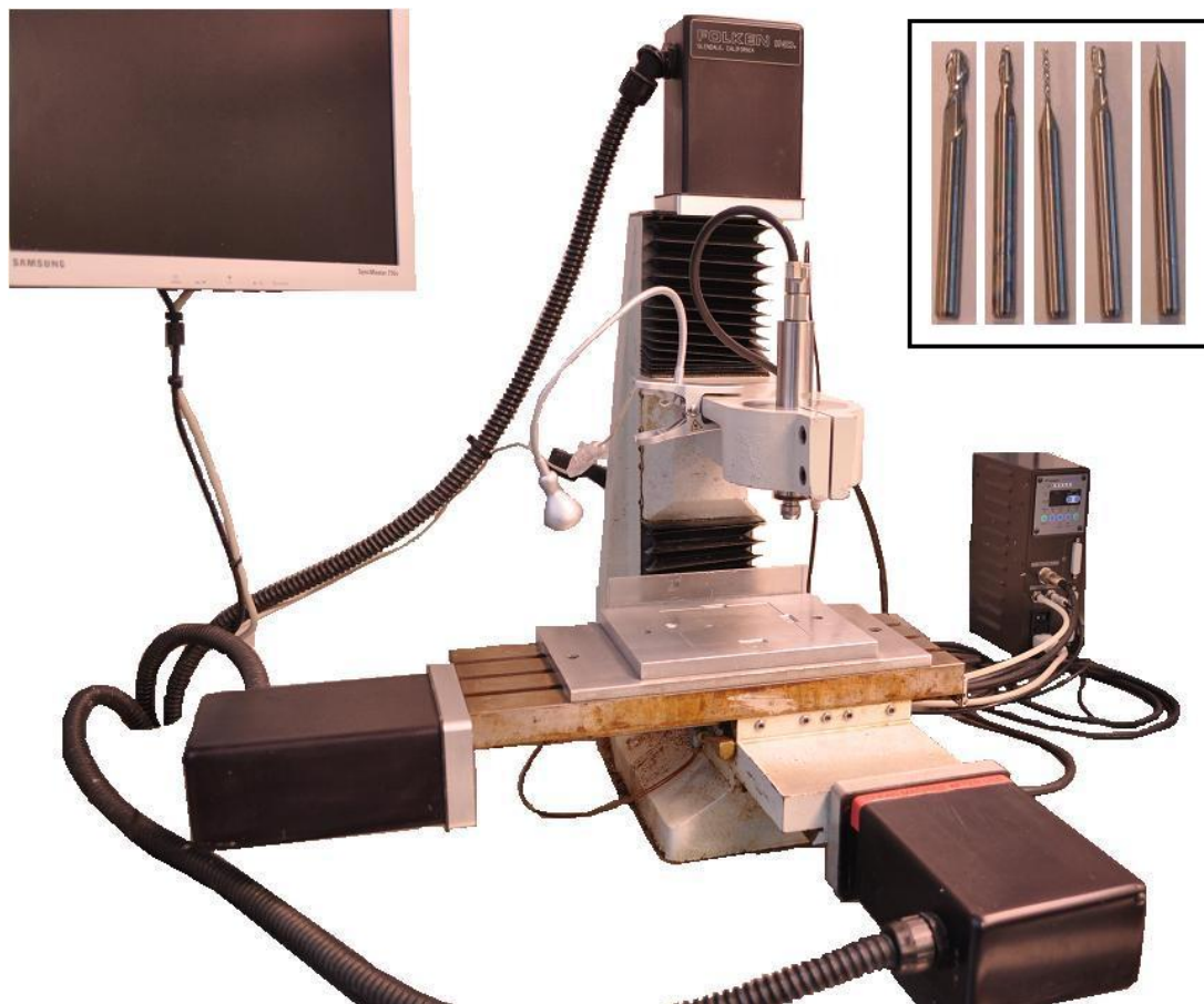
Figure 3.1: Micromilling machine. Inset shows tool bits used for micromilling.
