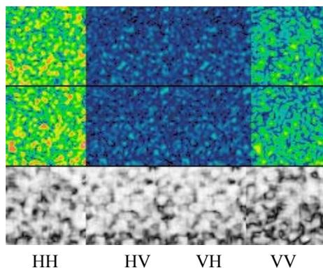
Figure 3. Simulated GB-SAR images of wheat for the 20cm baseline with no clutter motion and the resulting coherence image formed using a 5 by 5 window.
