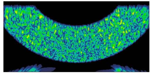
Fig. 6. Simulated static-case GB-SAR image using the distributed point scatterer model, for the parameters described in the preceding text. The image represents an area 20m in azimuth and 10m in ground-range. The features at the bottom corners are associated with range-ambiguity aliasing.
