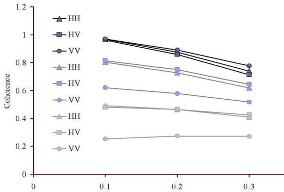
Fig 4. Effects of inter-aperture clutter motion on interferometric direct volume coherence by polarimetric channel. RMS wheat ear displacements are zero (top 3 curves), 0.7cm (middle 3) and 1.3cm (lower 3). VV returns come predominantly from the top of the canopy where displacements are greatest.
