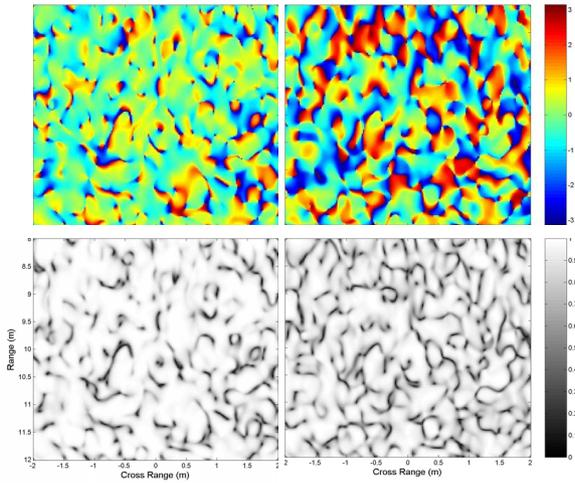
Figure 7. The top images show the phase stability  $\pm\pi$  between the static and moving cases for mean displacements (left) 0.124cm and (right) 0.375cm , respectively, for a 4m x 4m area centered at a range of 10m. The lower images are the respective coherence images, using a sliding 5 x 5 window, and displayed over a range 0-1.
