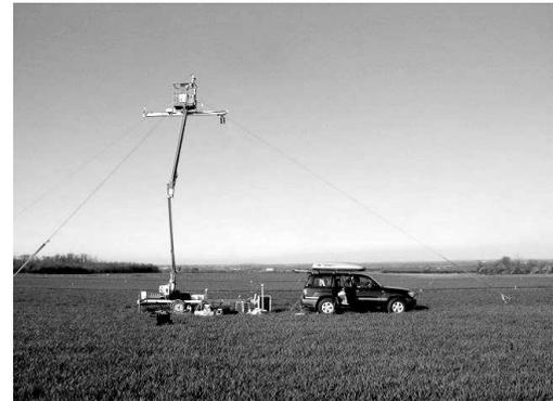
Figure 1. The deployed GB-SAR Outdoor System.
