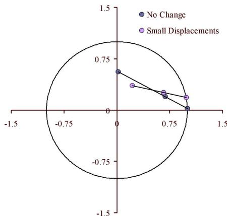
Figure 5. Effects of clutter motion on attempts to recover vegetation height and extinction using VV and HV coherence as volume and ground indicators respectively. Clutter motion shortens the extent of the sample in the complex coherence plane, and alters the recovered heights and extinctions.
