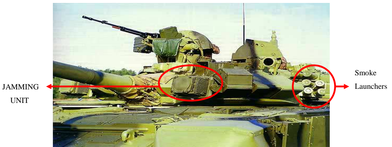
Figure 4 Shtor-1 employs a pair of electro-optical jammer
