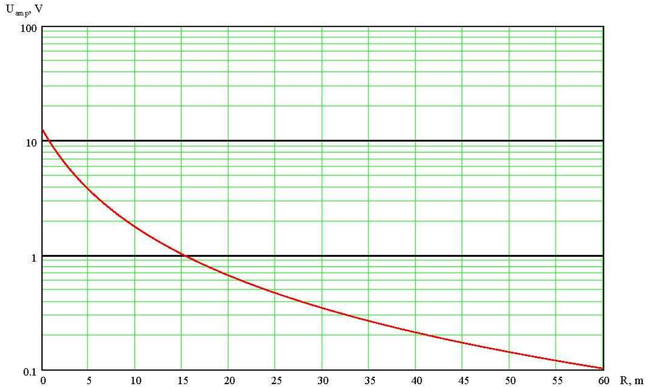
Figure 21 Amplifier output against range
