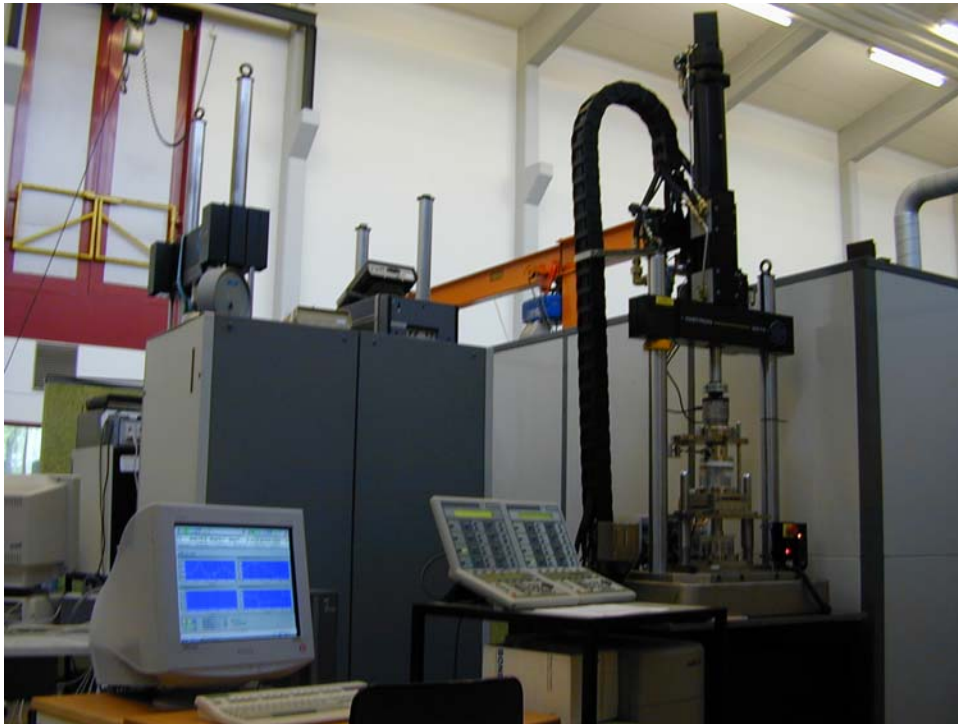
Fig. 2 Experimental set-up for simulating materials wear due to continued exposure to friction, pressure etc.
