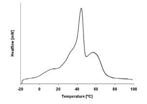
Figure 2. Thermal transitions of wheat straw wax determined by DSC.
