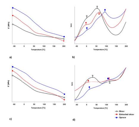
**Figure 1.** (a) Storage modulus (*E'*) and (b) loss factor (*tan*  $\delta$ ) of straw, extracted straw and spruce. The samples moisture content were 8.4 %, 8.3 % and 9.0 % for straw, extracted straw and spruce. c) Storage modulus (*E'*) and (d) loss factor (*tan*  $\delta$ ) of dry straw, dry extracted straw and dry spruce. It has to be noted that the scale on the y-axes (*E'* and *tan*  $\delta$ ) was adjusted for better comparison of the samples.
