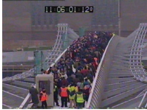
Figure 6: Crowd tests on the London Millennium Bridge (Shown with permission from Arup Partnership).
