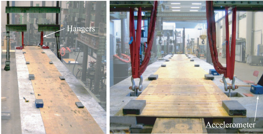
Figure 3.1: Suspended concrete platform at the laboratory of DTU Civil Engineering
