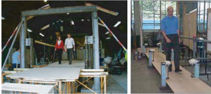
Figure 9: Platform tests commissioned by the French Road Directorate (left) and Arup (right), (Pictures from [75] and http://www.arup.com/millenniumbridge/. )
