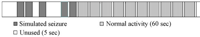
Fig. 6 – Diagram of the segmentation of the data strings from files containing simulated seizures. Between each segment a period of 5 s of data is left unused. Each normal activity segment lasts 1 min.
