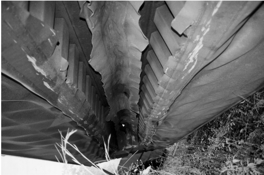
Figure 9.14: Frog's eye view of a double bottom deformed by a conical rock with a rounded tip. Example of how strong stiffeners on the longitudinal girders introduce hard points, early shell rupture and possibly bad energy absorption. From experiments conducted by the NSW, USA, [106].
