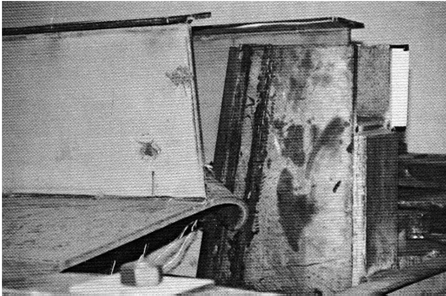
Figure 6.3: Cutting of a 20 mm thick plate by a wedge, [10].
