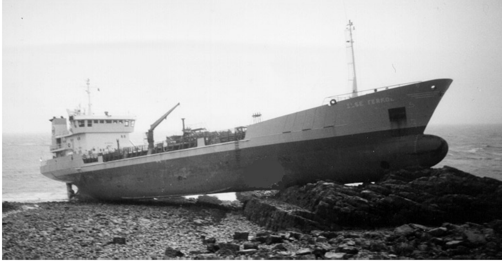
Figure 3.6: Grounding of the Else Terkol in the Bristol Channel. The tide is 8 m.
