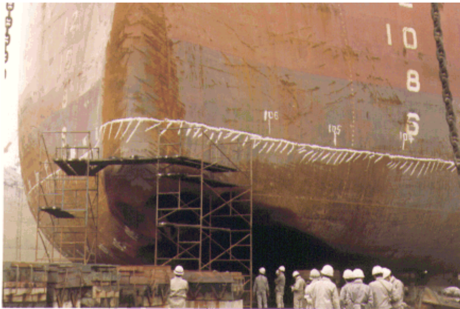
Figure 10.8: Picture of damaged hull of single hull VLCC. From [63].
