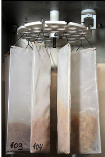
Figure 4.4. Climate chamber with conic device to seal the gap to the balance lead-through.
