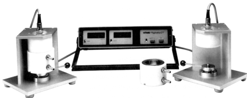
Figure 3.2. Probe for accurate measurements of the equilibrium humidity inside small samples.
