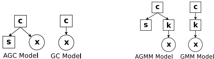
Figure 5.1: The left part of the figure compares the Probabilistic Graphical Models of the Gaussian Classifier (GC) and the proposed Aspect Gaussian Classifier (AGC). Consult e.g. [57] or [49] for an introduction to Graphical Models. C denotes the genre class random variable, S denotes the song index and X is the feature vector. Round circles represent continuous variables, while squares represent discrete variables. The right part of the figure compares the graphical models of the Gaussian Mixture Model (GMM) and the proposed Aspect Gaussian Mixture Model (AGMM).
