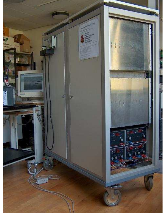
Fig. 8. The experimental RASMUS scanner. RASMUS has 128 transmitting channels and 64 receiving channels with 2:1 multiplexing. Arbitrary waveforms can be transmitted and the individual received channel data can be recorded for later processing.
