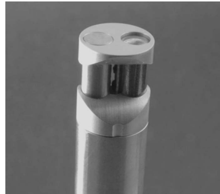
FIG. 2. A Microflow 1/2 in. sound intensity probe. The particle velocity sensor can be seen on the solid cylinder to the right; the electret microphone is mounted inside the other cylinder.
