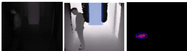
Figure 2. Tracking a person in a dark room. left) gray image, middle) depth image and right) plane view with cluster ellipse of the person. The blue overlay region indicates the location of a door.
