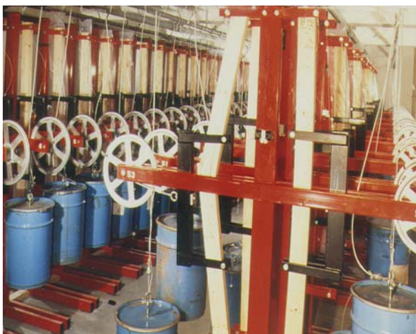
Fig. 1 Long-term test rigs to accommodate two boards each
