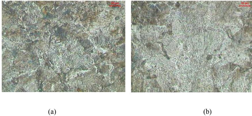
**Fig. 2.** Scanning electron micrograph of Fe-3%Mn-0.8%C specimen sintered at (a) 1120°C and (b) 1250°C in 100% nitrogen atmosphere. Note larger overall grain size of the 1250°C sintered material.
