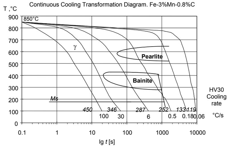
Fig.4. Continuous Cooling Transformation Diagram for Fe-3Mn-0.8C.
