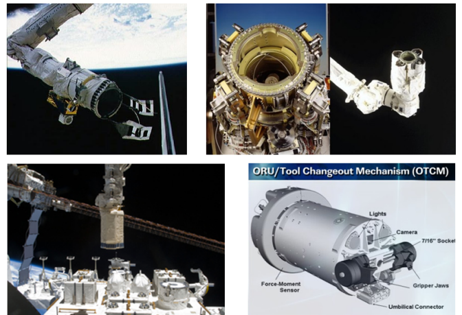
Fig. 4. Existing standard interfaces: Top left: EE on SRMS (Courtesy of NASA), Top right: LEE on SSRMS (Courtesy of NASA), Bottom left: JEMRMS (Courtesy of JAXA), Bottom right: OTCM (Courtesy of NASA).
