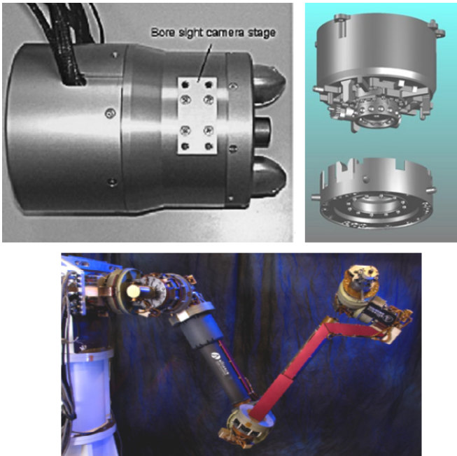
Fig. 5. Different standard interfaces: Top left: JAXA EE (Courtesy of JAXA), Top right: CTED (Courtesy of ESA), Bottom: RSGS interface (Courtesy of MDA).
