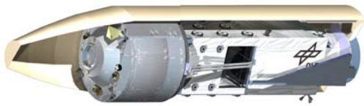
Fig. 6: Free Flyer in stowed configuration inside the expected Ariane 6-4 fairing.
