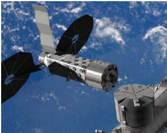
Fig. 4: Fully equipped Orbital-Hub's Free Flyer with deployed photovoltaic and radiator wings.
