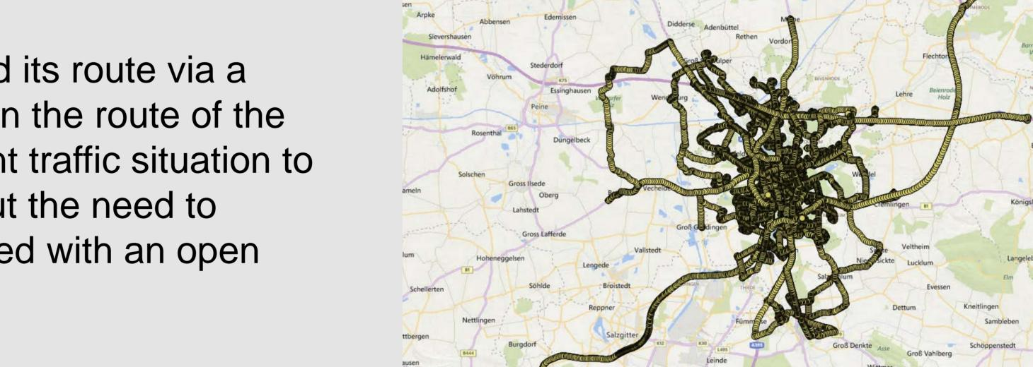
The emergency vehicle sends its current position and its route via a Car2X communication application. The traffic lights on the route of the emergency vehicle will be set according to the current traffic situation to let the emergency vehicle pass all traffic lights without the need to violate a red light. The traffic evaluation was performed with an open source traffic simulation called SUMO.
