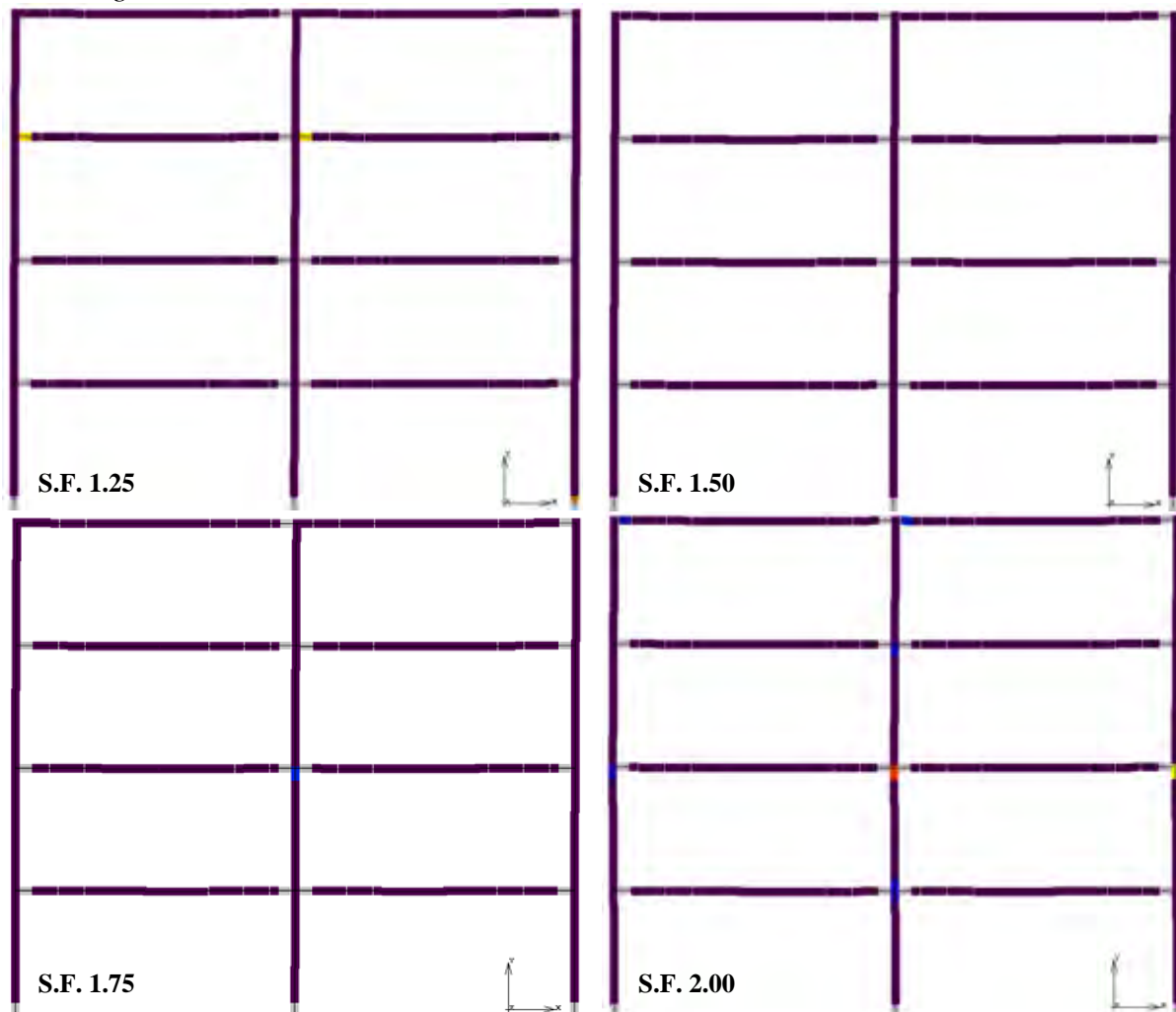
Figure 9-31: Development of plastic hinge mechanism for S.F. 1.25, 1.50, 1.75 and 2.00 (290xa).
