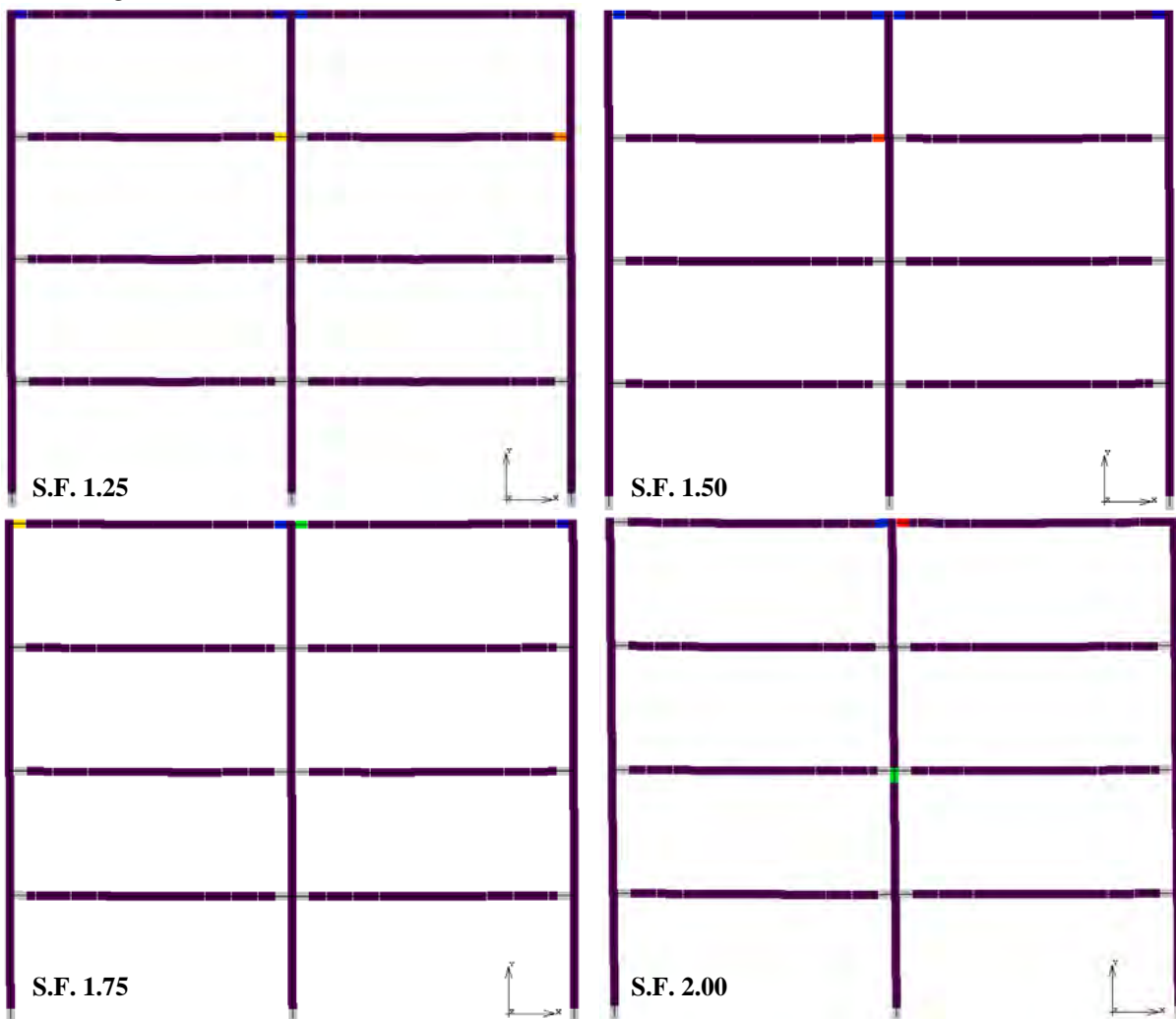
Figure 9-37: Development of plastic hinge mechanism for S.F. 1.25, 1.50, 1.75 and 2.00 (612xa).
