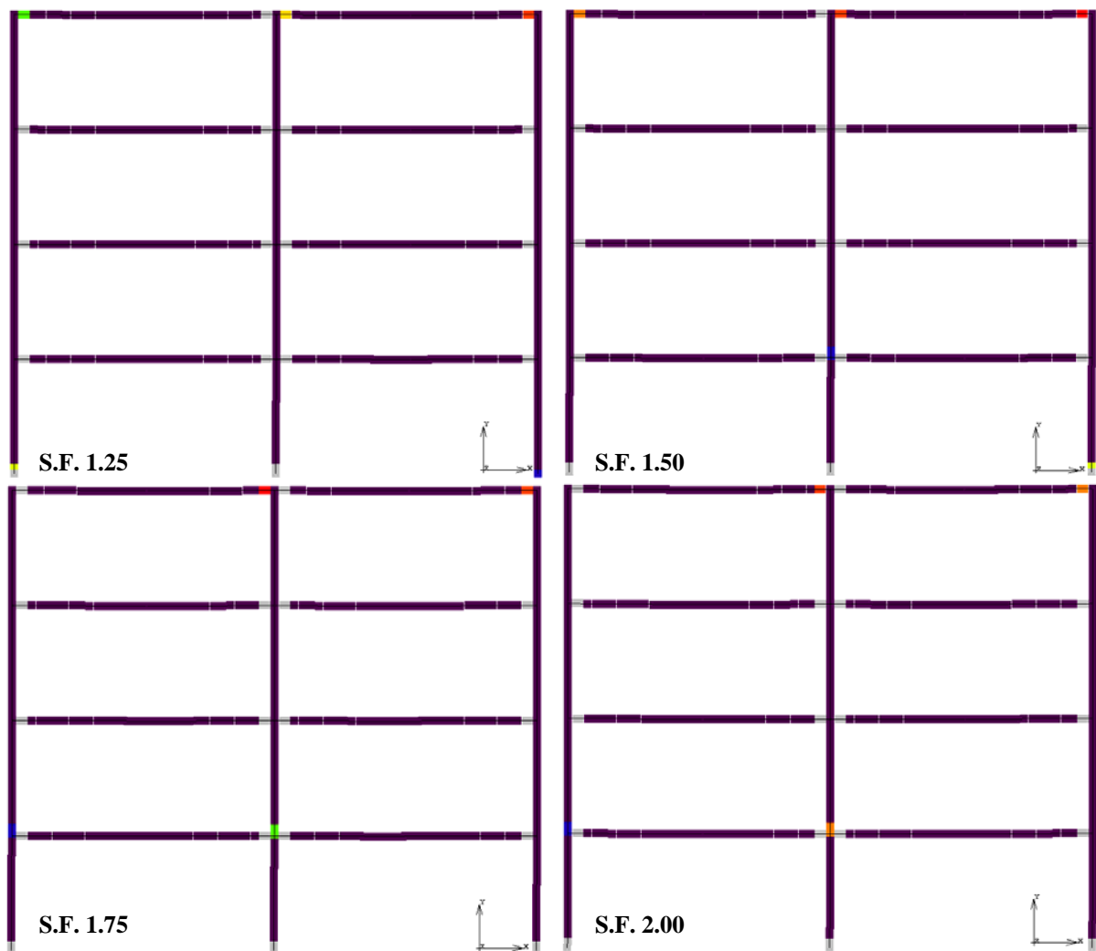
Figure 9-43: Development of plastic hinge mechanism for S.F. 1.25, 1.50, 1.75 and 2.00 (5850xa).
