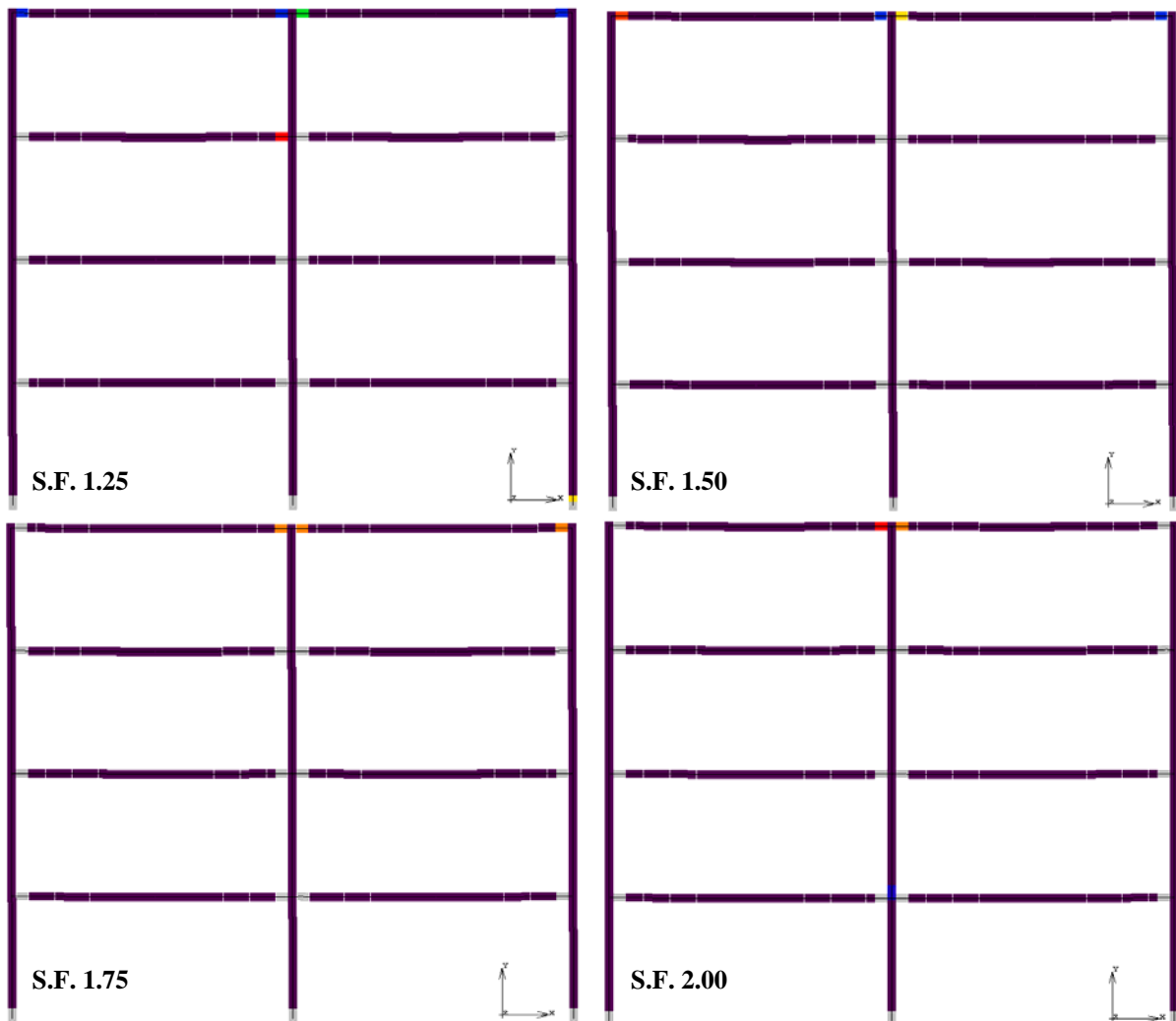
Figure 9-41: Development of plastic hinge mechanism for S.F. 1.25, 1.50, 1.75 and 2.00 (1726ya).
