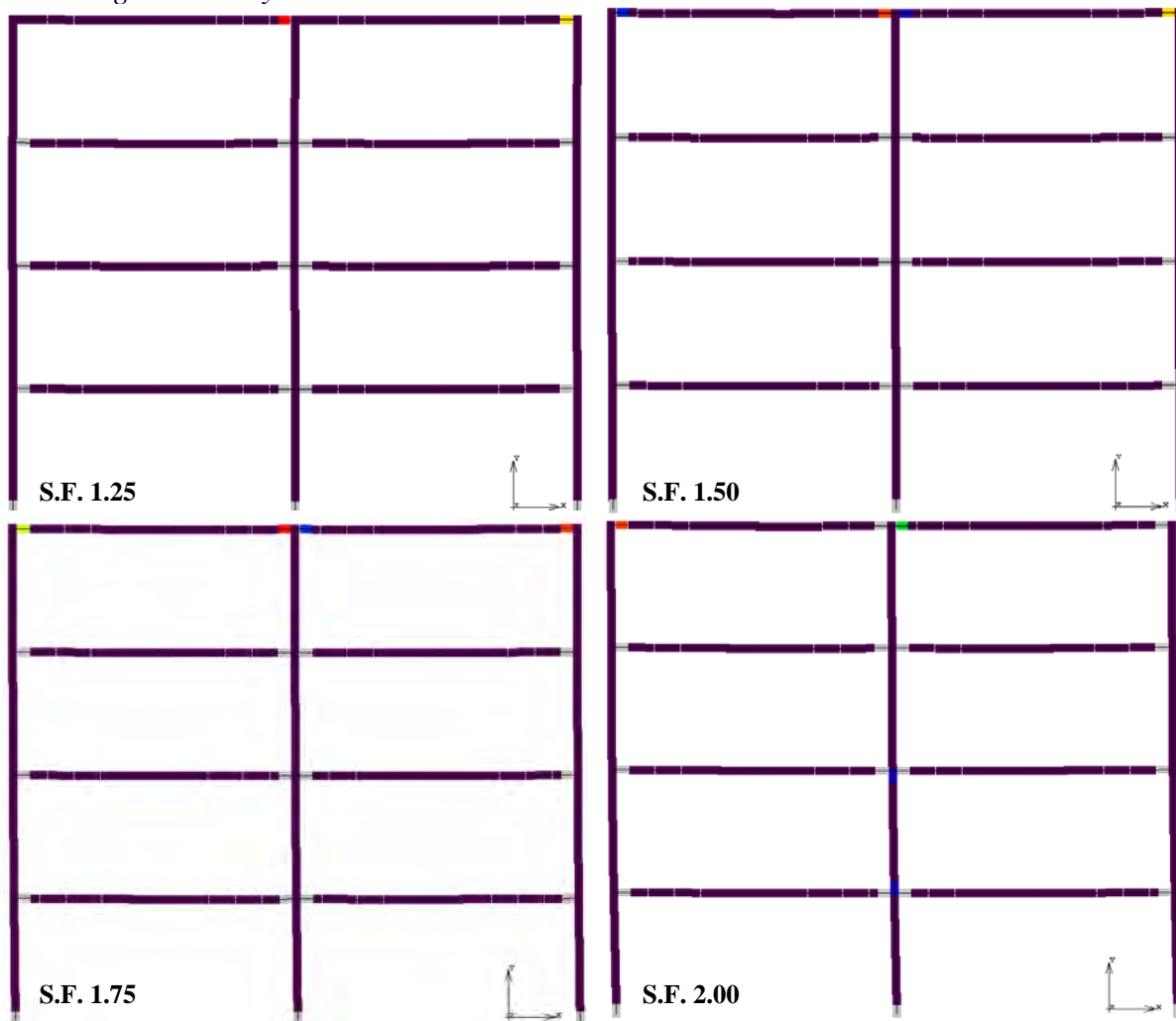
Figure 9-35: Development of plastic hinge mechanism for S.F. 1.25, 1.50, 1.75 and 2.00 (6142ya).
