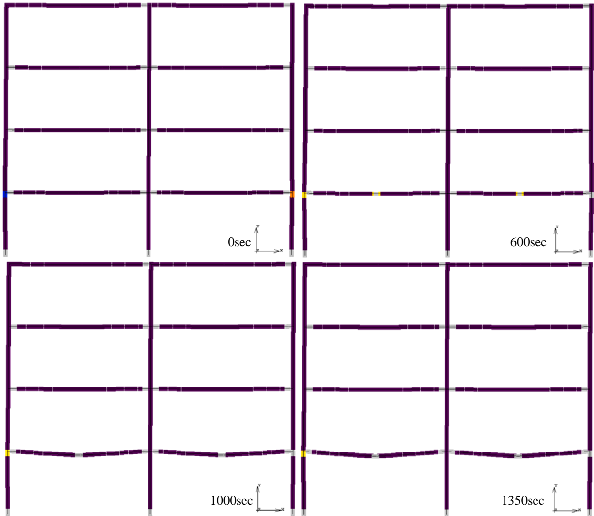
Figure 11-12: Deformed shape of the structural system and the equivalent plastic strain distribution (Layer 1) during the FAE loading for scenario E290xa-1.50-FISO.
