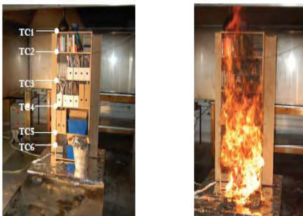
Figure 8-7: The bookshelf setup and the burning stage.
