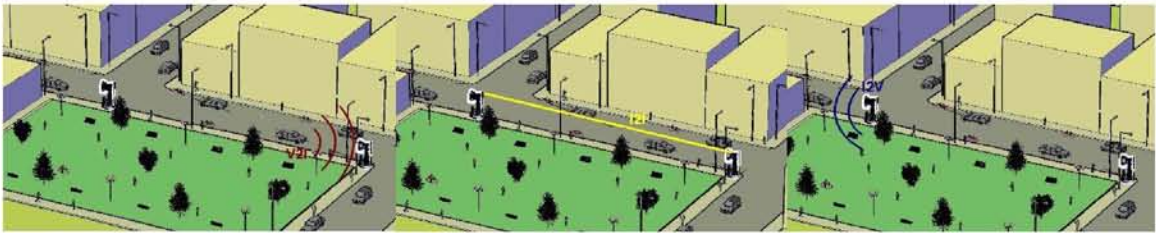
Figure 7.2: Application example of ErouVe System. A. Vehicle approaching intersection sends a beacon message to RSU B. Infrastructure-to-infrastructure communication for information exchange C. Vehicle receives routing instructions.
