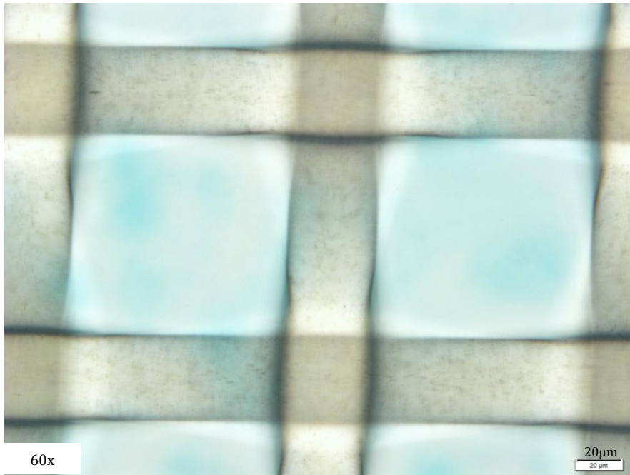
Fig. 4.26 – Focused mesh on the active layer side of a FO membrane (60x)
